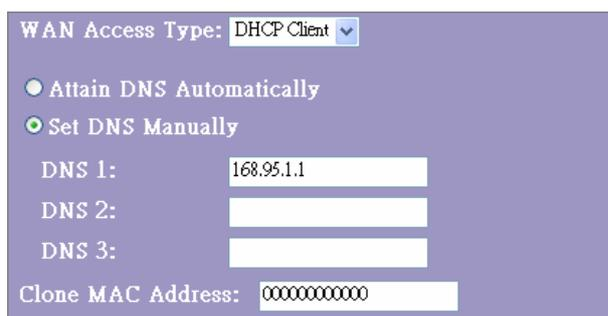
The screenshot shows the WAN Interface Setup form in DHCP Client Mode. The 'WAN Access Type' is set to 'DHCP Client'. The 'Attain DNS Automatically' radio button is selected. The 'Set DNS Manually' radio button is unselected. The fields are filled with the following values: DNS 1: 168.95.1.1, DNS 2: (empty), DNS 3: (empty), and Clone MAC Address: 000000000000.
