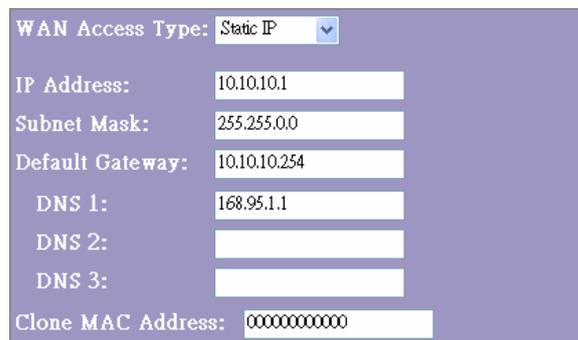
The screenshot shows the WAN Interface Setup form in Static IP Mode. The 'WAN Access Type' is set to 'Static IP'. The fields are filled with the following values: IP Address: 10.10.10.1, Subnet Mask: 255.255.0.0, Default Gateway: 10.10.10.254, DNS 1: 168.95.1.1, DNS 2: (empty), DNS 3: (empty), and Clone MAC Address: 000000000000.
