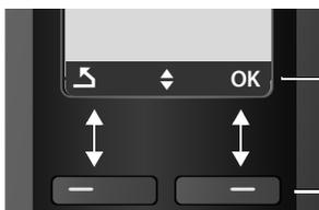
Current display key functions are shown in the bottom display line.
